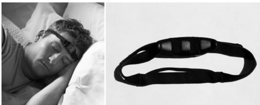
Figure 1. The headband, about the size of a tennis headband, is comprised of three dry silvercoated fabric sensors and a sealed plastic enclosure containing electronics for signal sampling and transmission to a base station for processing.
